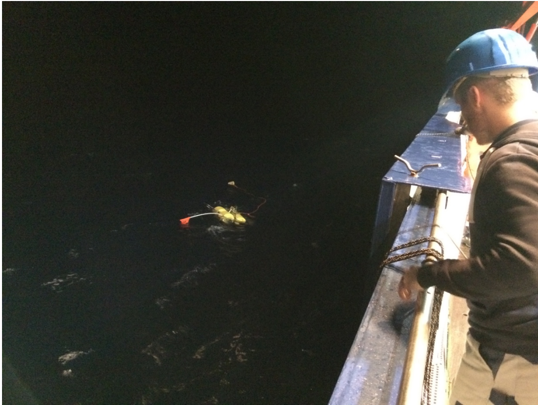
OBS waiting for its recovery on the starboard side of RV Maria S Merian. Photo: Y. Xia, GEOMAR
